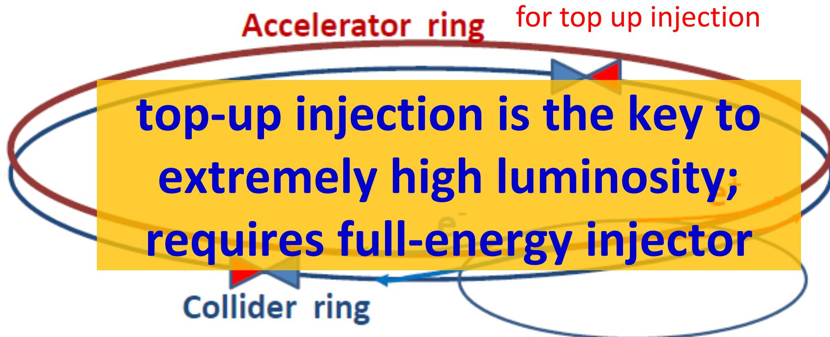
short beam lifetime ( $\sim \tau_{\text{LEP2}}/40$ ) due to high luminosity supported by top-up injection (used at KEKB, PEP-II, SLS,...); top-up also avoids ramping & thermal transients, + eases tuning
