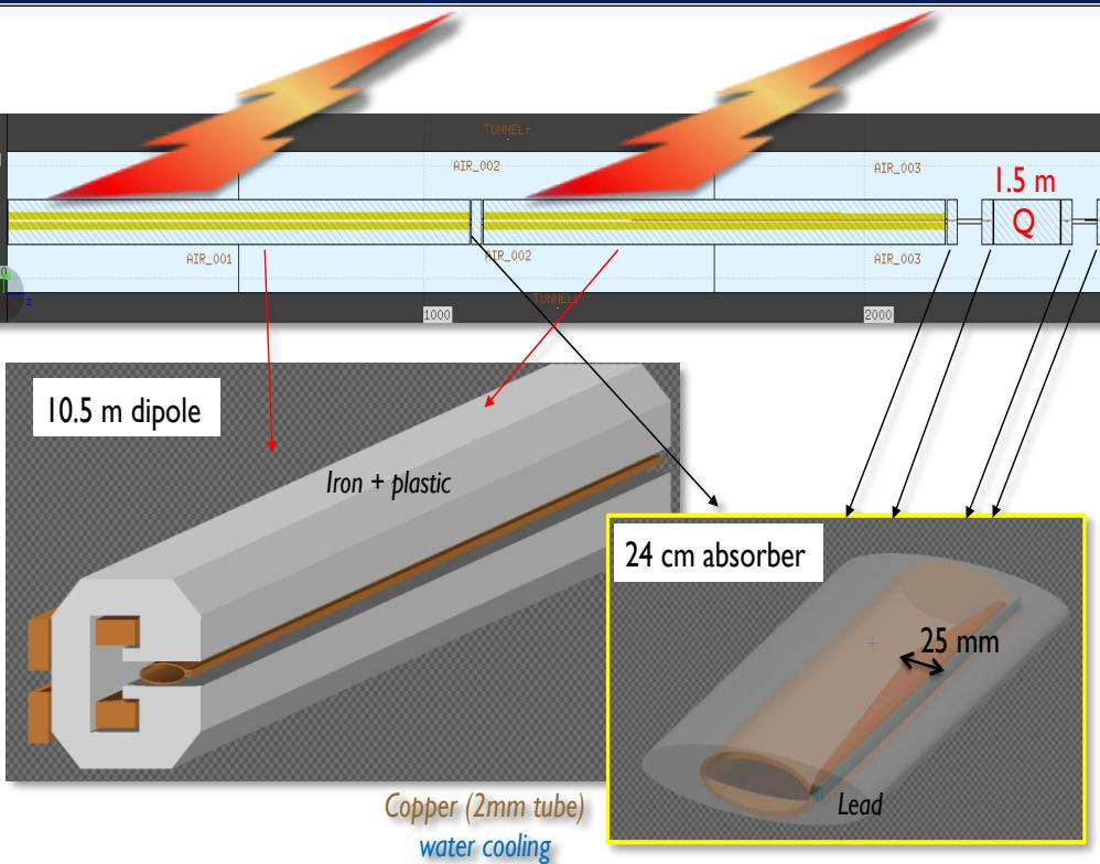
FLUKA geometry layout for half FODO cell, dipoles details, preliminary absorber design incl. 5 cm external *Pb* shield
