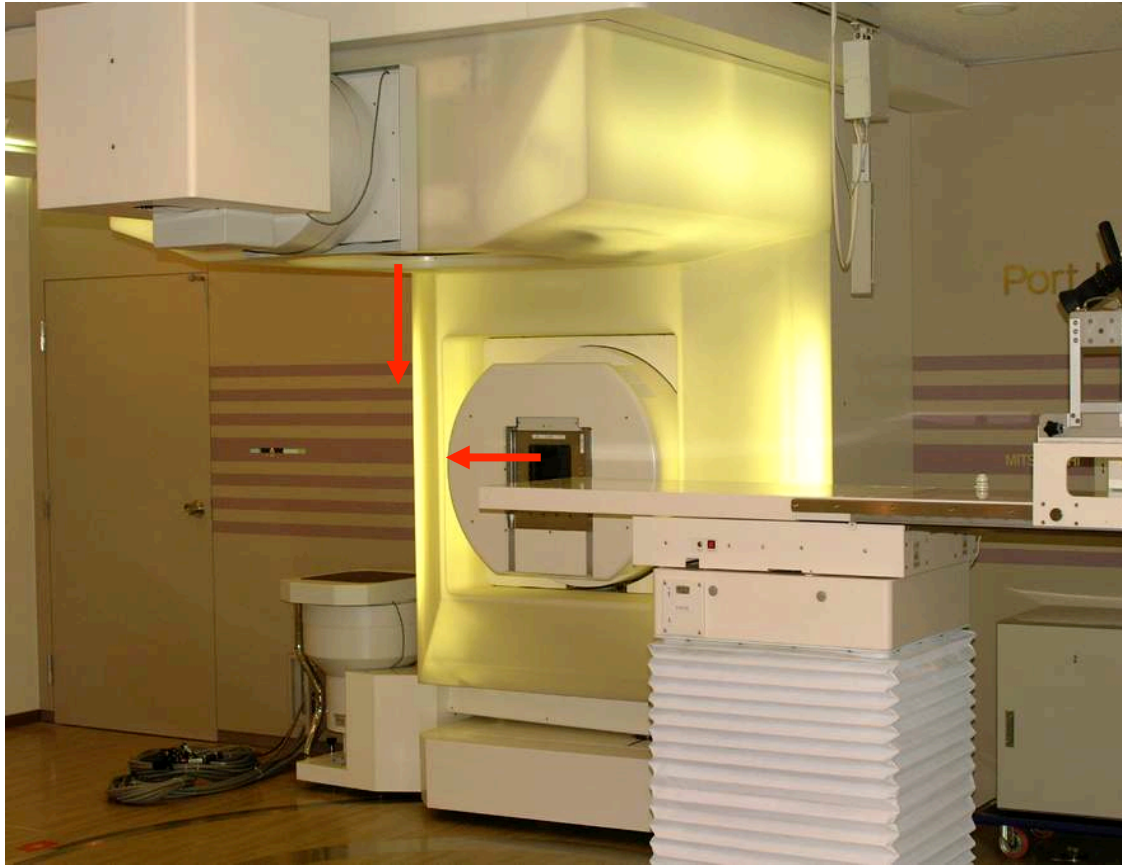
Horizontal & vertical beam lines
