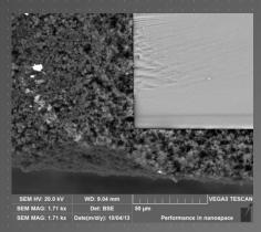
A SEM photograph of planar sensors with enriched Boron sputtered on the surface
