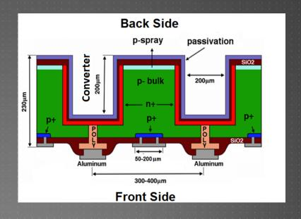
Planar sensor with guard ring and sputtered converter on the top
