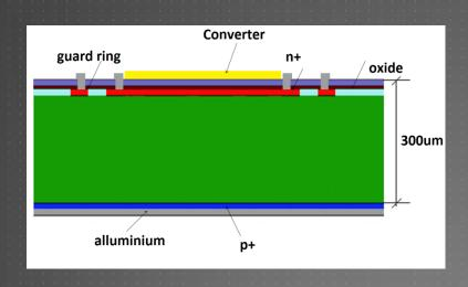
3D sensor schematic crosssection (not to scale), with values of the main geometrical parameters with all the contacts are on the front side.
