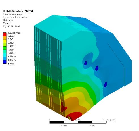
(Deformation due to magnetic forces at 5T)
