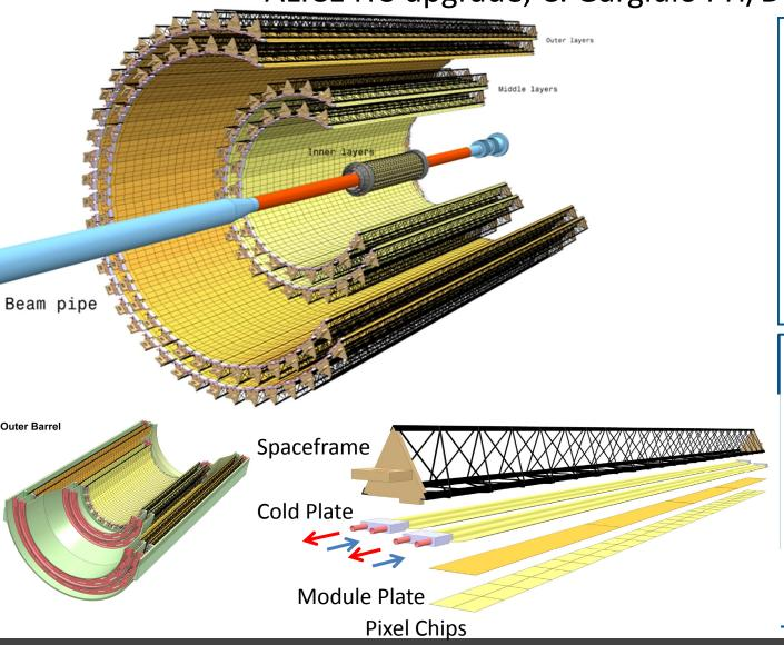
Inner Barrel (IB): 3 layers pixels
