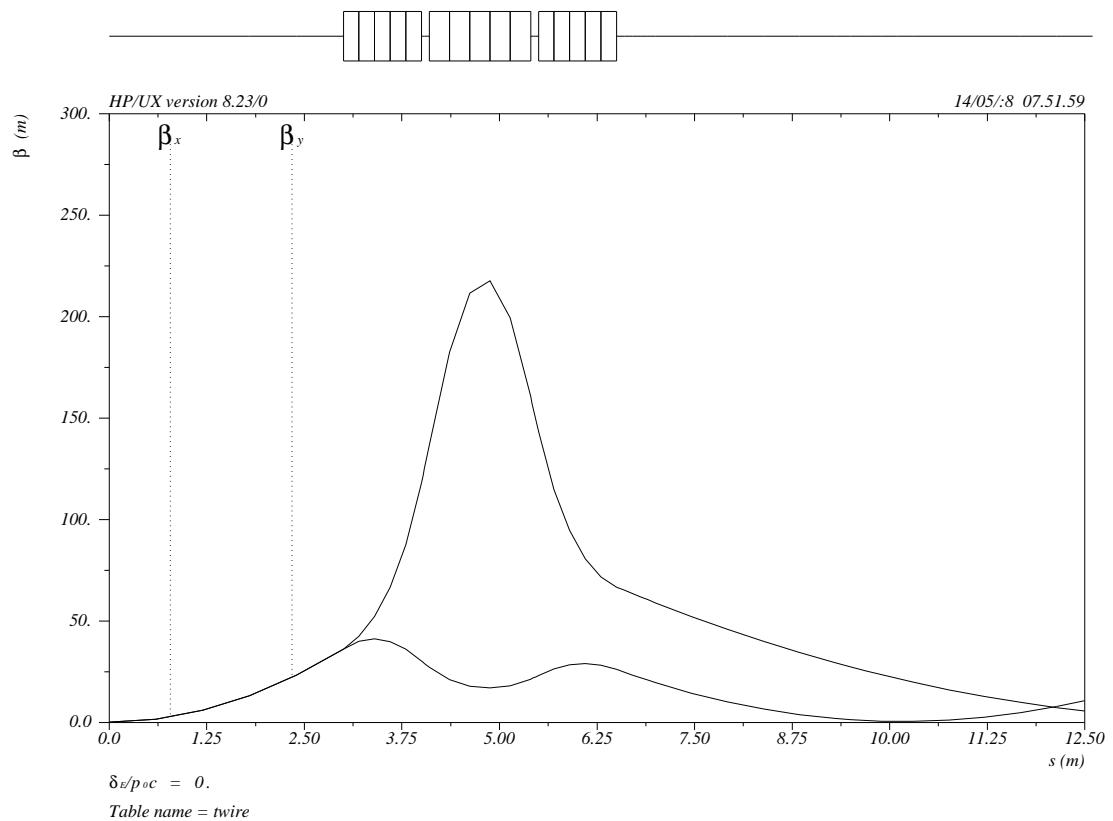
Low- $\beta$  triplet (warm or cold), common to both beams.
