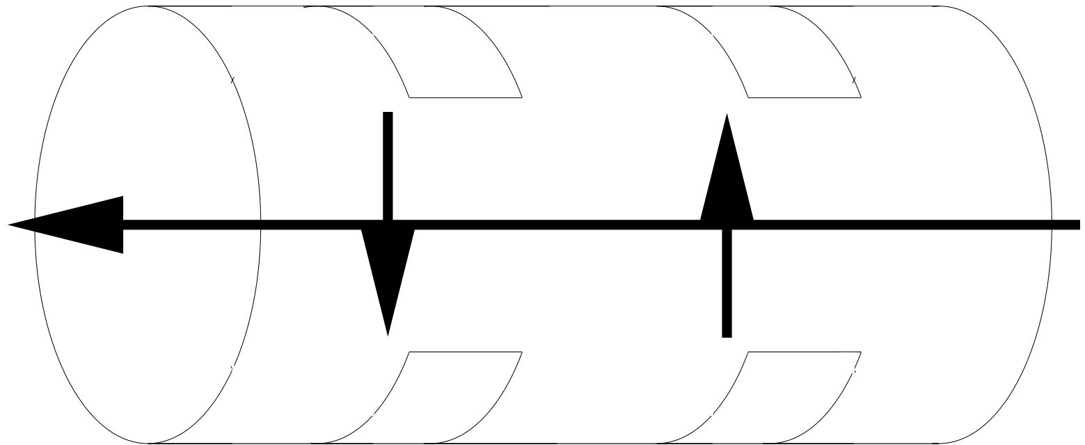
Detector-integrated dipoles: dipole coils as part of detector solenoid
