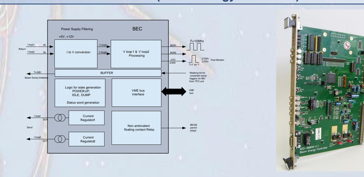
The BEC module interfaces the BEM and BEI modules to external systems through redundant fail safe connections. It produces the dump request signal that is fed to other systems for any failures detected within the BETS.
