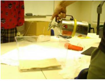
5. PREPARE THE ICE - Now take the dry ice and put it into the wooden box. Make sure to use thick gloves (the ones for handling heavy things or heavy winter gloves) and safety goggles when handling the ice. The temperature of the ice is  $-78^{\circ}\text{C}$ ! Finally put the box with the metal plate on the bottom on the ice. Now your chamber is ready to detect particles tracks !!!
