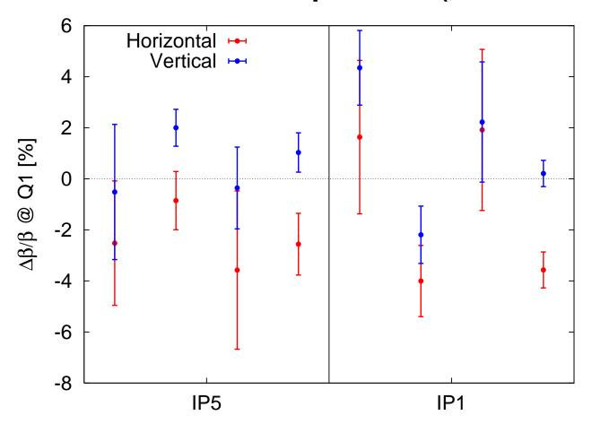
$\beta$ -beating below 5% at Q1s. Resolution of few % is not enough for a  $\beta^*$  measurement (IP1/IP5 luminosity imbalance  $\approx$ 0).
