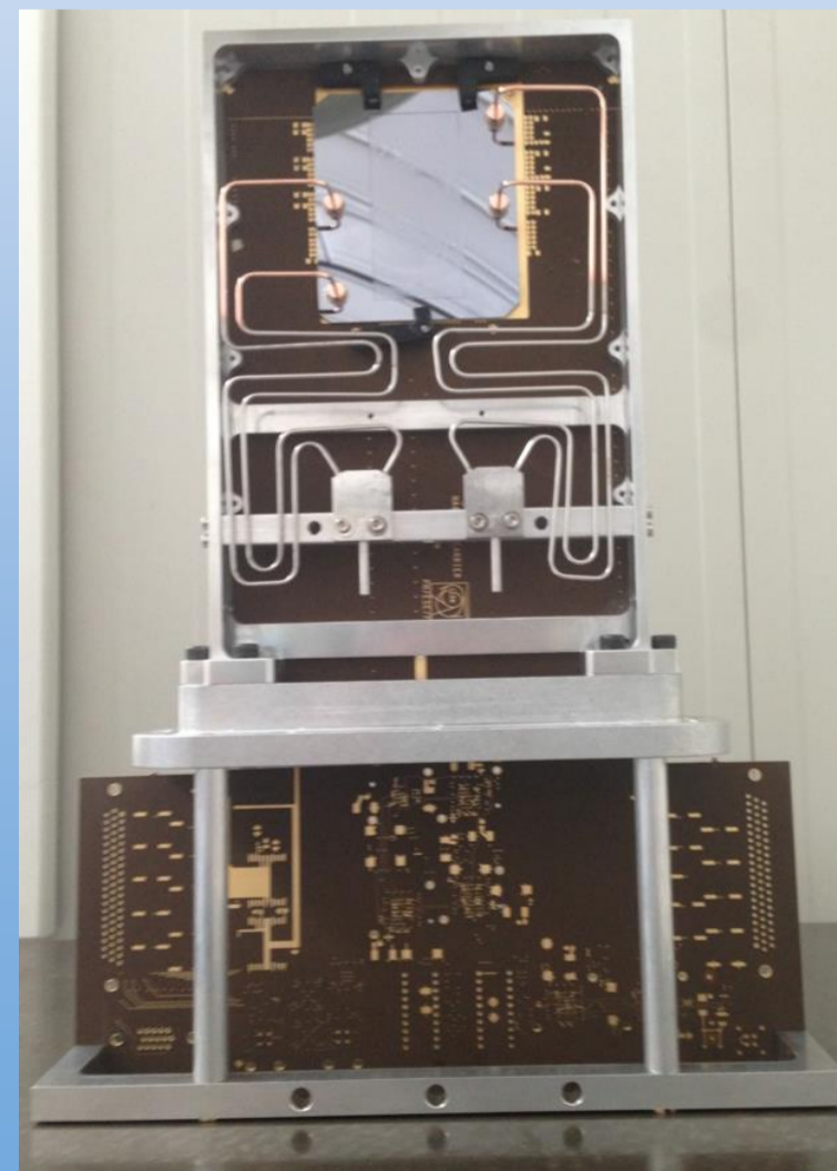
Jig for precision gluing of detector on pre-equipped \mu -channel device
