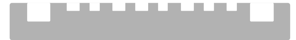
DRIE etching of channels
