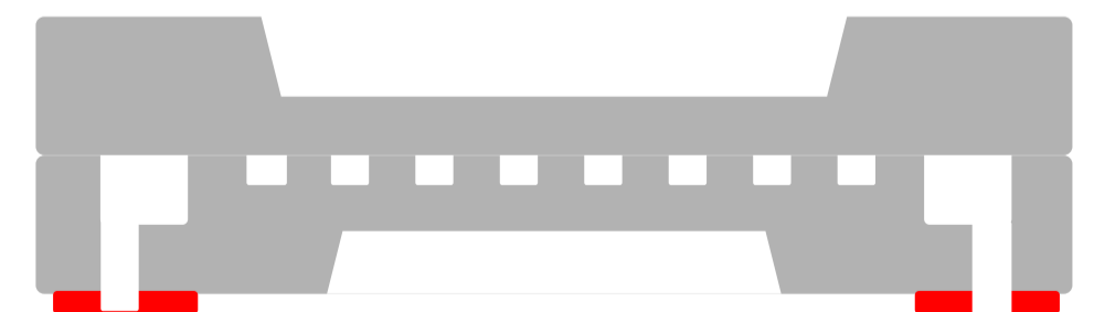
Metalization for soldering connectors
