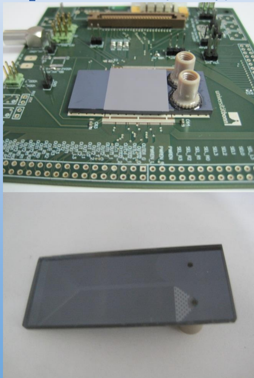
CO 2 micro channel prototype for FE-I4.
