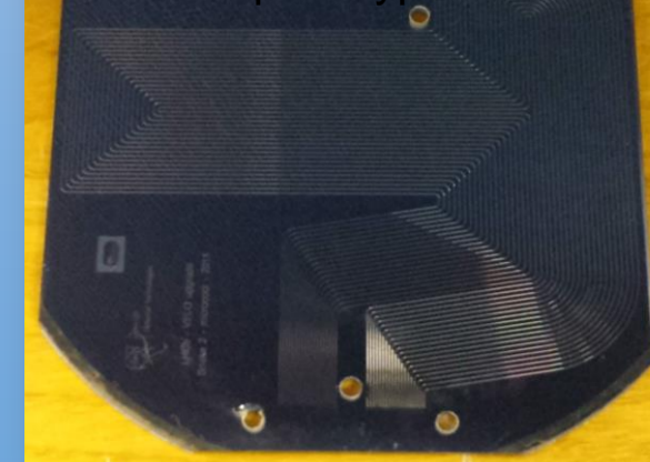
Si-Pyrex micro channel substrate prototype
