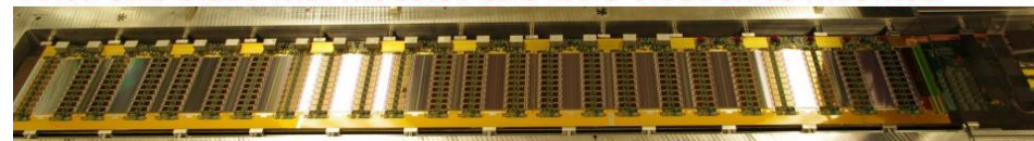
A full size stave with modules and EOS electronics mounted
