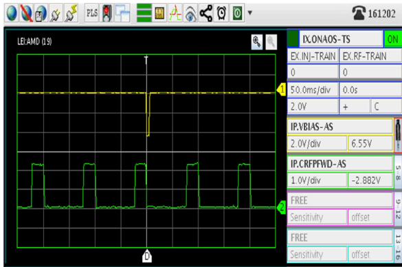
Figure 3: Analog signal of the GTS ion source of Linac3, showing the ion source pulsing with a bunch spacing of 100\text{ms} and a bunch duration of 200\mu\text{s} .
