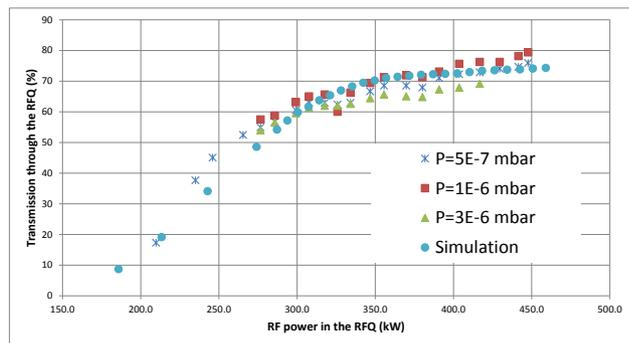
Figure 6: Transmission vs. RF power in the RFQ for different LEBT pressure. The nominal RFQ power is 400kW. Simulations in light blue dots.
