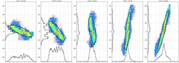
Figure 3: Transverse phase space profile for increasing solenoid field, units of mm and mrad.
