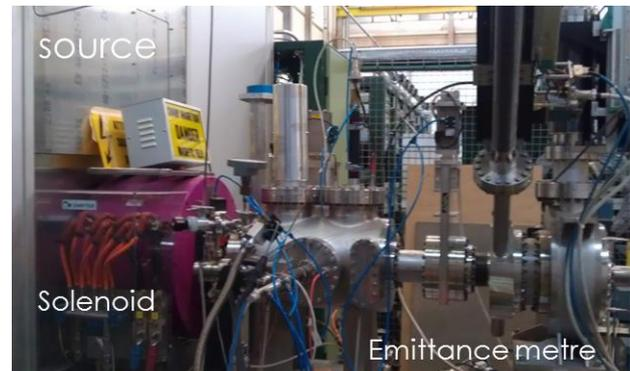
Figure 2: Set-up for emittance measurements at 45 keV.
