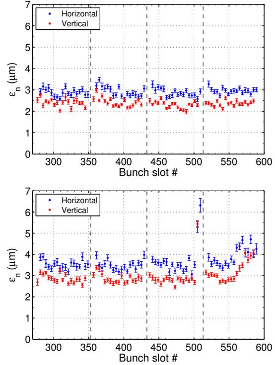
Figure 3: Bunch by bunch emittances measured at the SPS flat top for  $4 \times 72$  bunches of the 25 ns LHC beam with intensities at injection of  $N \approx 1.35 \times 10^{11}$  p/b (top) and  $N \approx 1.45 \times 10^{11}$  p/b (bottom).
