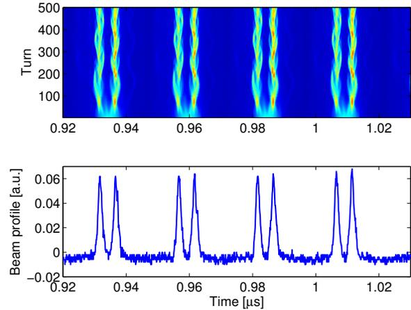
Figure 4: Evolution of the longitudinal beam profile in the SPS during the splitting at injection for the production of the doublet beam (top) and longitudinal bunch profiles of the doublet beam measured 1 s after injection (bottom).
