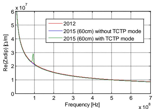
Figure 3: Impact of the 100 MHz mode of the 8 TCTP and 1 TCSG per beam on the real part of the horizontal impedance of the current LHC model for  $\beta^*=60$  cm (in green), compared to the case without this “TCTP mode” (in blue) and to the 2012 impedance model (in red).
