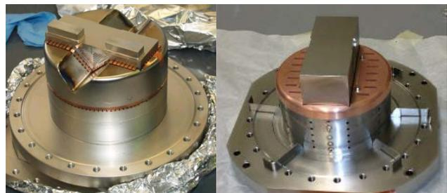
Figure 2: Shielding of ATLAS-ALFA (left) and consolidated TOTEM (right) roman pots installed during LS1 to improve the impedance (courtesy ATLAS-ALFA and TOTEM).
