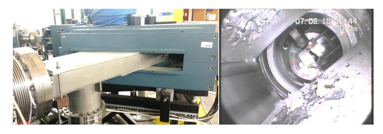
Bending vacuum chamber. Complex design (not to CERN methods).
