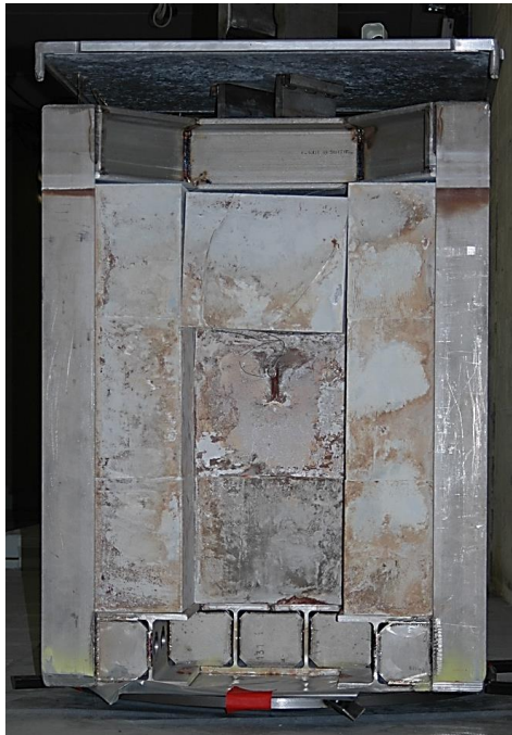
Damaged and oxidized target #1
