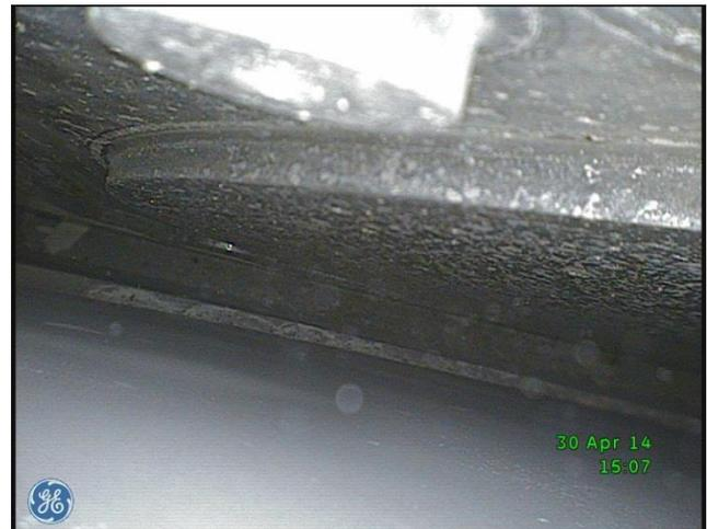
Figure 2. Initial signs of corrosion at the target neutron window
