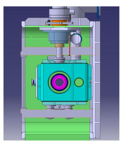
Interferences between cavity helium vessel and the cryostat wall
