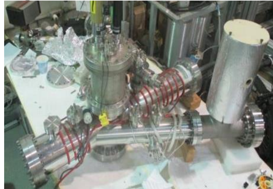
Primary ion source 3-way switchyard To connect primary source, ToF, and emittance meter to the EBIS
