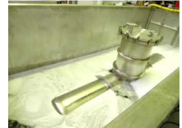
Helium vessel cleaning at manufacturer's premises
