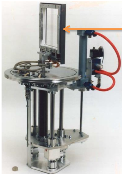
Wire grid (NTG) at high-rad area
