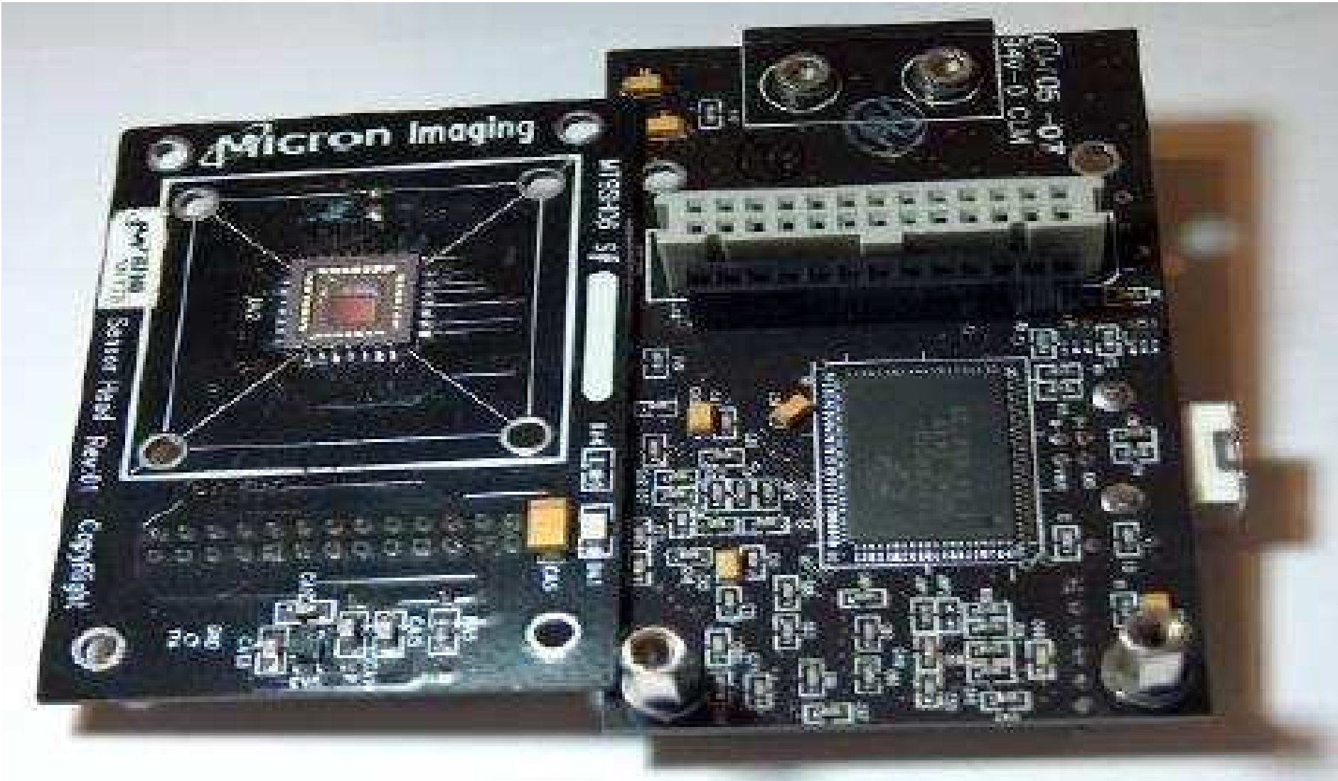
MT9V11 Si CMOS sensor (left) and MT9SH06 readout board (right) [1].
