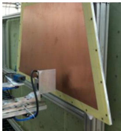
Panel Flatness/Planarity measurements (Laser based)
