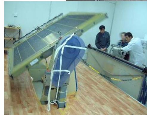
Wire winding on rotating table (China)
