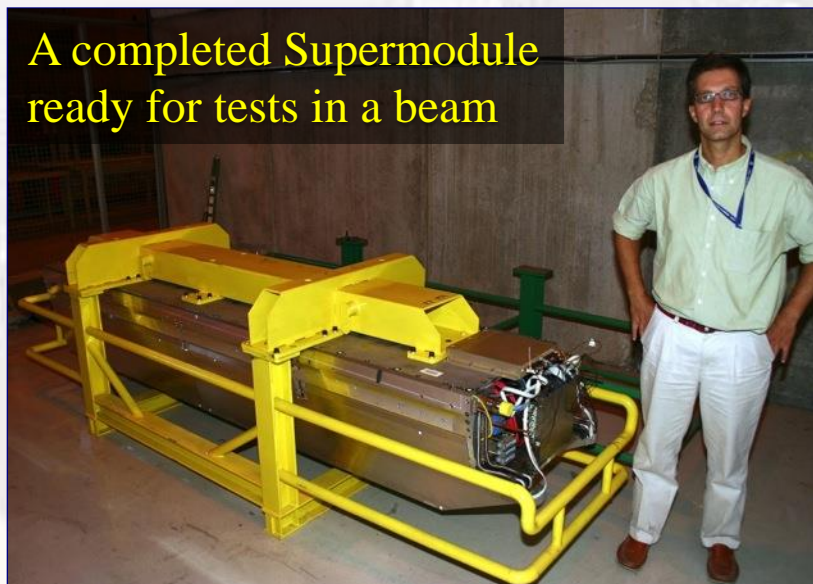
An ECAL Module of 400 crystals
