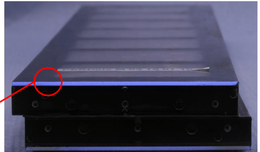
PERDaix: 860 mm (L) x 32 mm (W) bi-layer module in stereo geometry.
