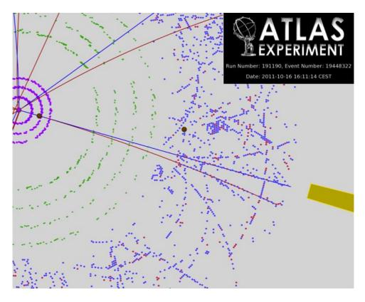
,Isolated' photons not in jets Information about direction Converted photon  $\gamma \rightarrow e^+e^-$ In tracking chamber + deposition
