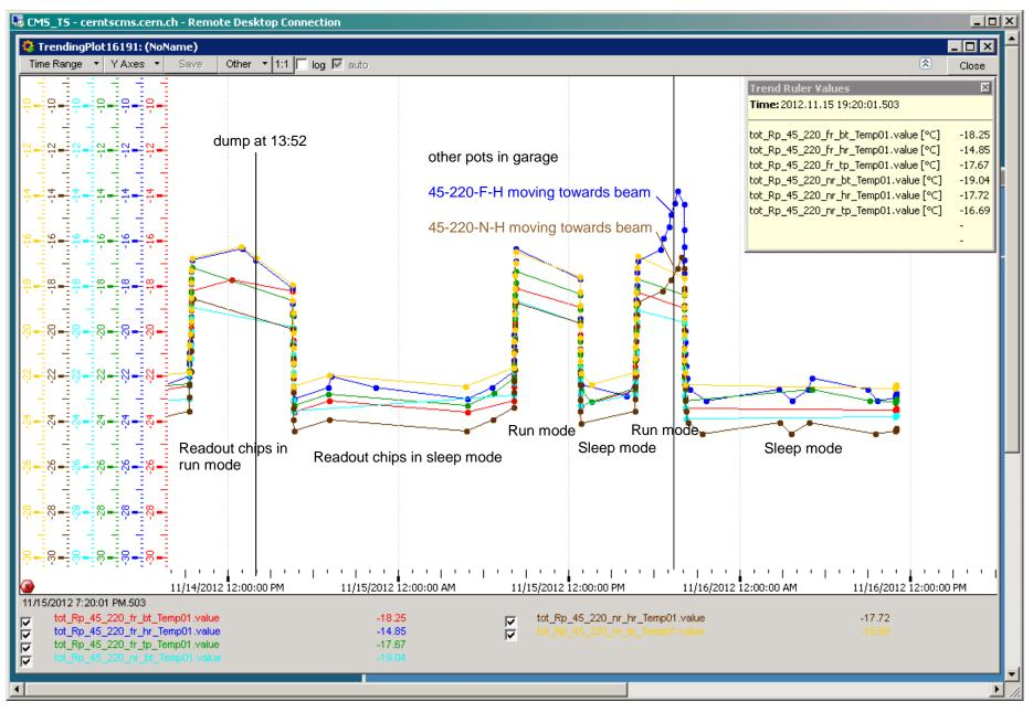
Main temperature effect from chips changing to run mode; small additional increase (3 deg.) from pots moving very close to the beam. UFOs cannot be resolved.
