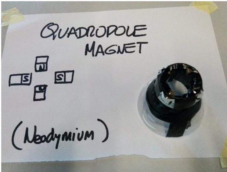
Handmade Quadrupole Magnet
