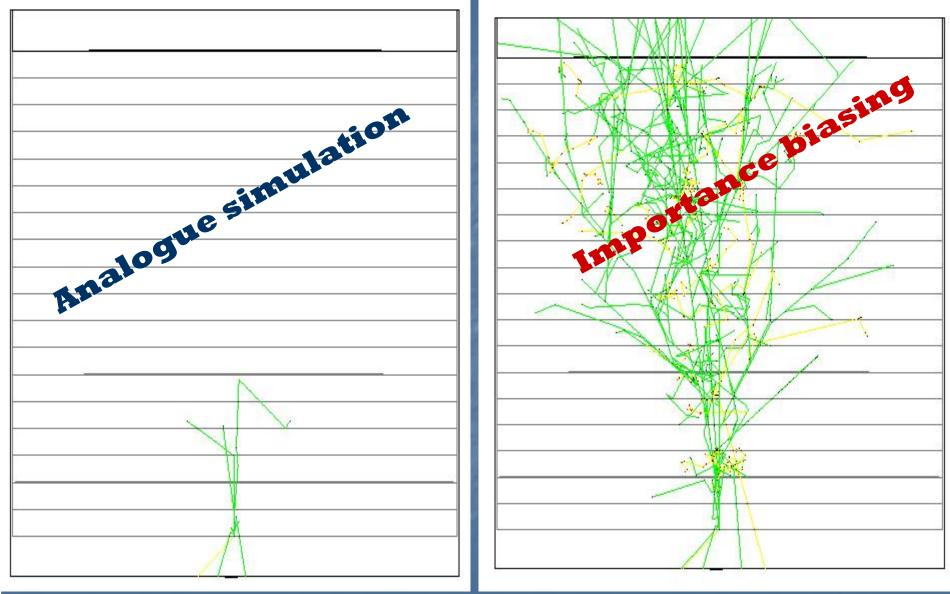
**10 MeV neutron in thick concrete cylinder**
