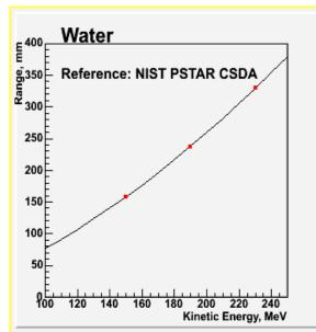
Ranges of proton are obtained in the simulation by switching off all processes except for ionization process.
