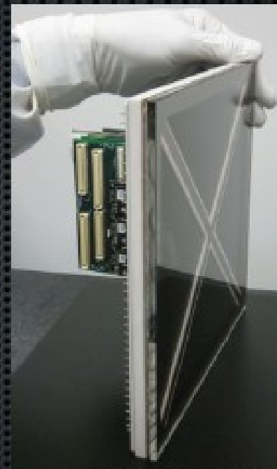
Berkeley SSL detector system - ceramic body LAPPD
