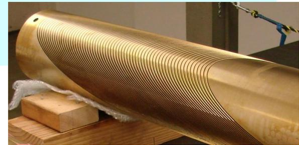
Spiral channels are cut into a cylinder.
