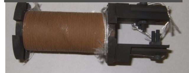
OP 2-layer coil; conductor length=11 m; nGimat insulation
