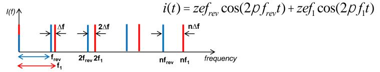
• Spectral density of the  $n^{\text{th}}$ -band of N particles with random initial phase and a revolution frequency spread  $f_{rev}$ + $\Delta f/2$ :
