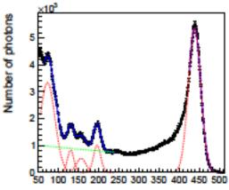
Am-241 energy spectrum measured by one beer can radiation detector constructed at the course
