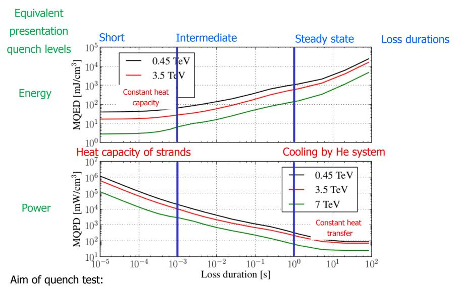
How much of beam intensity could impact on equipment and not quench a magnet
