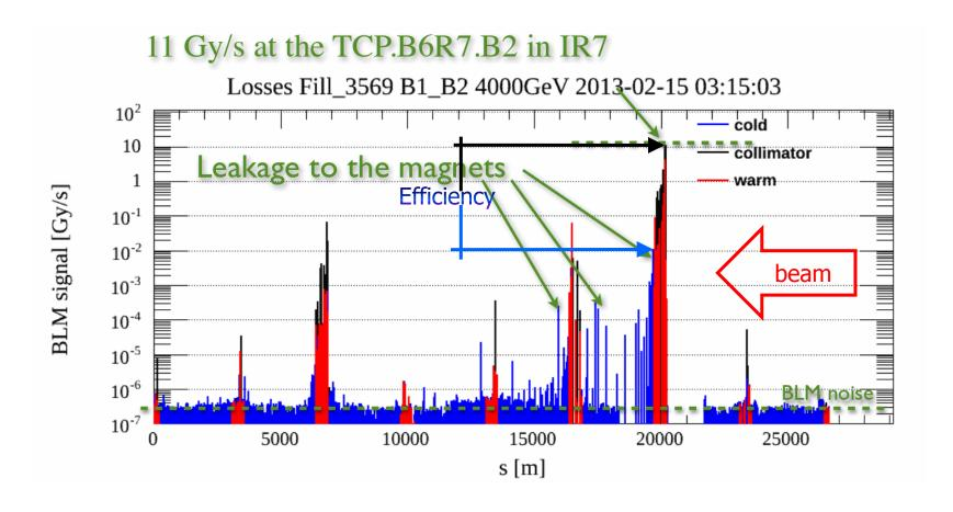
Determination of efficiency needed to plan upgrade requirements for collimation system
