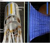
Antiproton annihilation into nuclear fragments and pions (MIP), observed at AEgIS (left). The scintillating fiber detector (right) detects the pions which are emitted when antiprotons annihilate on the surface of the vacuum vessel. The detector is used to measure antihydrogen production (right).
