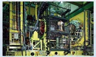
UA2 was a custom built setup around the beam pipe. UA2 had electromagnetic and hadronic calorimeters to detect electrons and hadrons, but could not measure particle charges except for limited regions where the W decay asymmetry was maximal. There was no muon detector.
