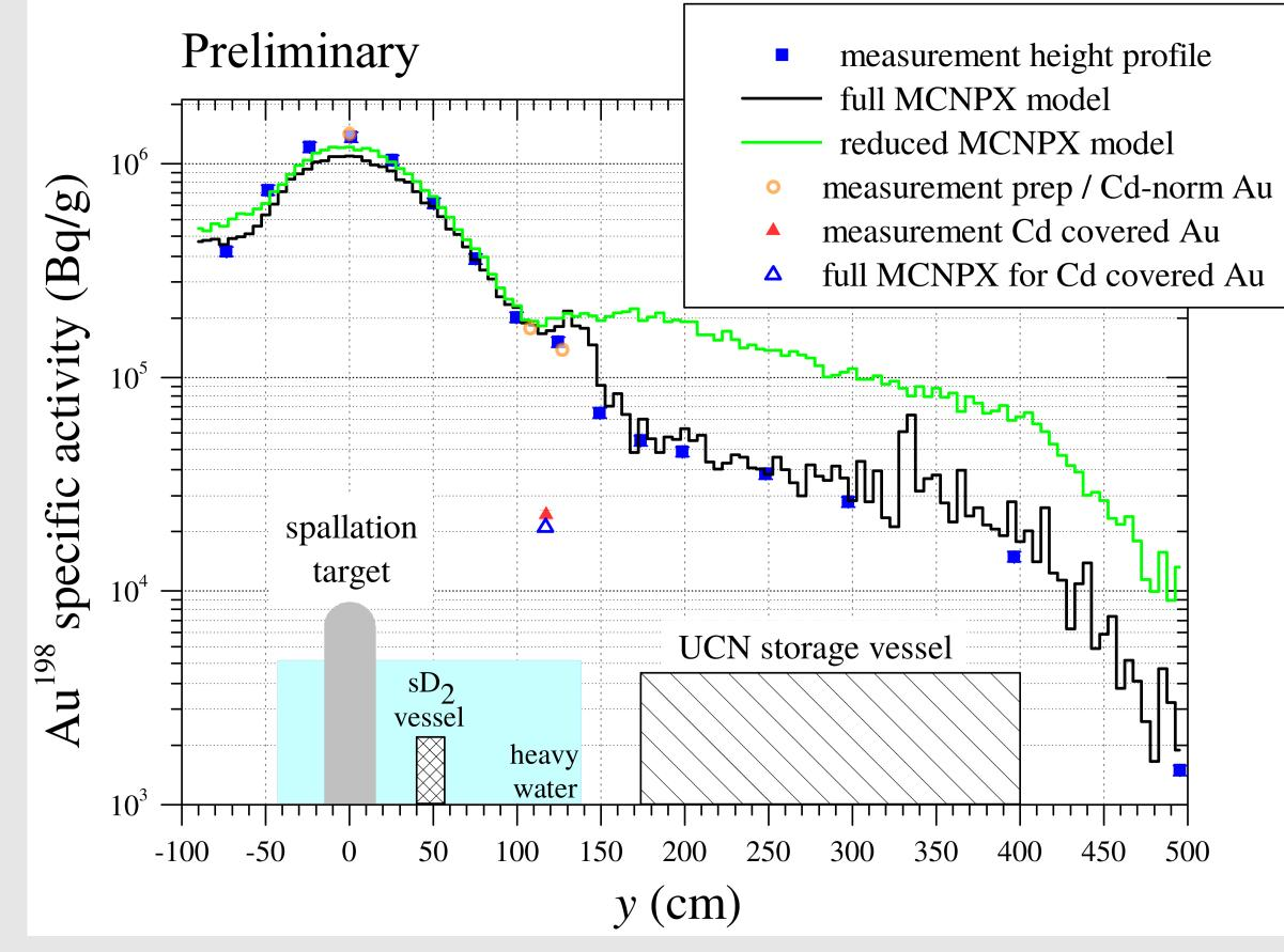
Measurement and simulation agree, which shows that the production of thermal neutrons in the target and  $D_2O$  moderator assembly are well understood.
