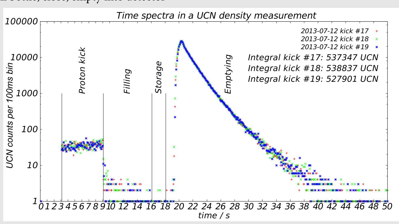
A density of 30 UCN/cm<sup>3</sup> was measured, taking into account transmission losses of the detector window. This places the UCN source at PSI among the best performing UCN sources in the world.
