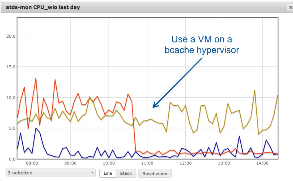
SSD block level caching sufficient for IOPS and latency demands.
