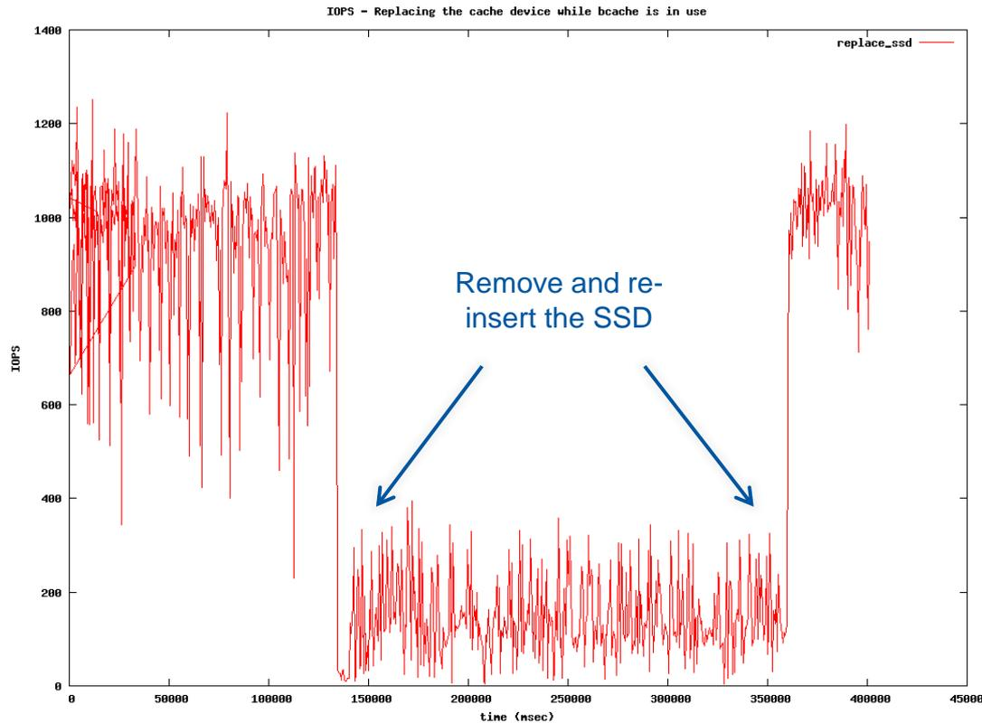
Simulate SSD wear-out replacement procedure:
