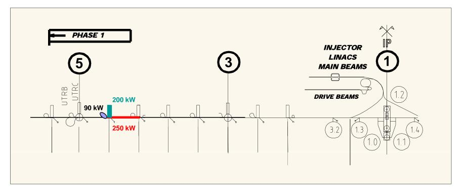
Heat dissipation in the tunnel: 250 kW / DB sector 1250 kW between two shafts Corresponding air flow: Delta T°C = 28-18 = 10 °C 370 000 m3/h -> 5 vol/h To be Optimised ...
