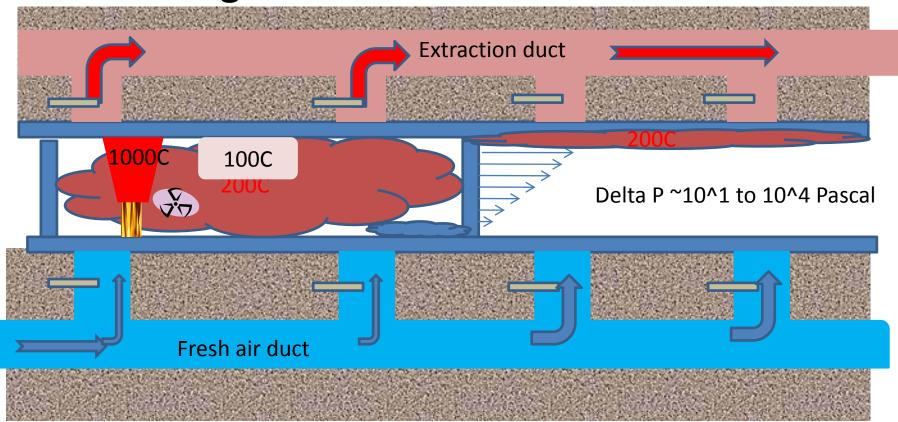
The natural overpressure of fire can be contrasted by overpressurizing the side compartments
