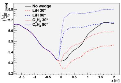
"Standard MICE beam" 6 mm transverse emittance Large 90 mm longitudinal emittance 25 MeV energy spread 200 mm dispersion at the wedge
