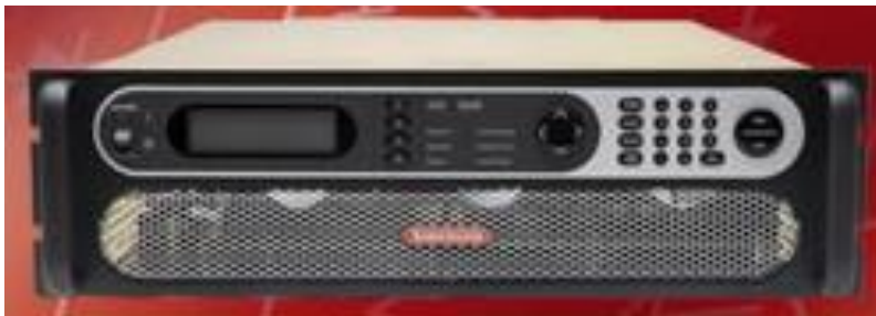
FC - Sorensen 250A power converter (main)
