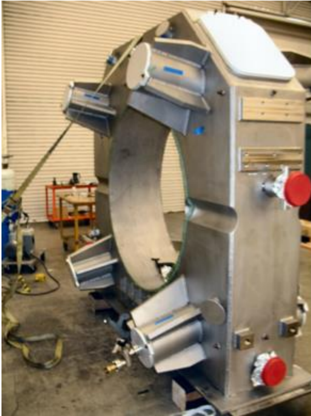
• Cryostat vacuum leak check
