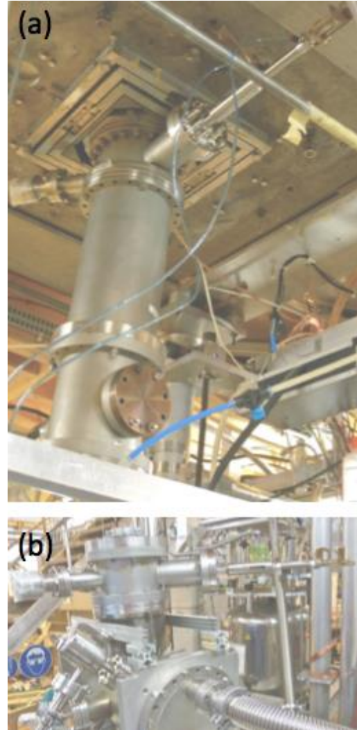
Fig. 3: (a) Optics chamber between the lower preparation and upper precision Penning traps. (b) Leak test of the upper part of the chamber shown in (3a).
