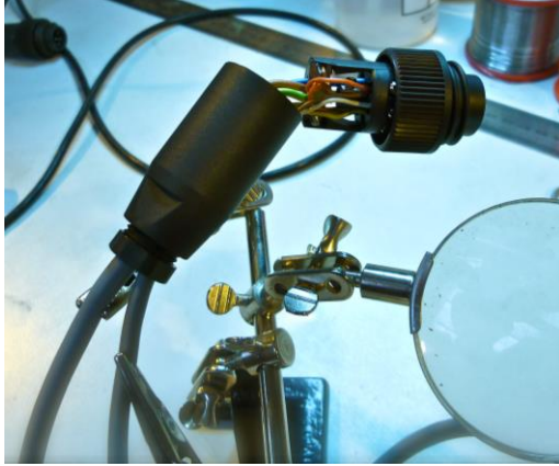
Fig. 2: Pin wiring for valve actuator plug.
