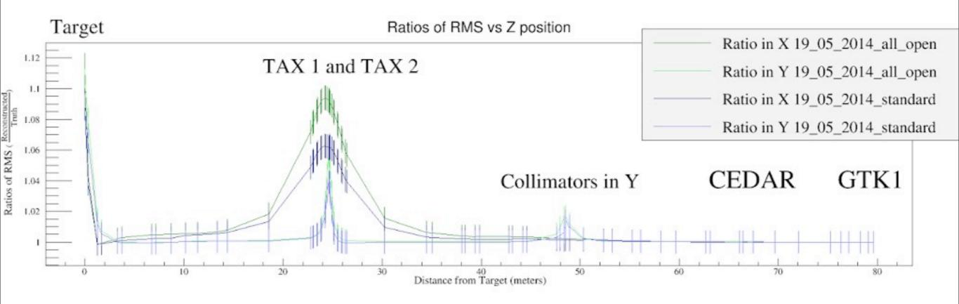
Expectation from observation with standard beam-line elements is correct. The removal of stopped tracks immediately at the given element reduces the information gained in the divergence of the beam spot.
