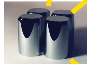
Array of 4 HPGe coaxial N type crystals
