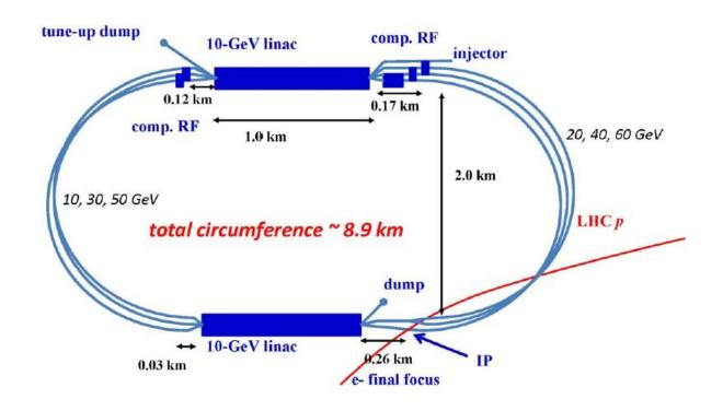
LHec; A Large Hadron Electron Collider at CERN; sections 8.1.2, Fig 8.5.
