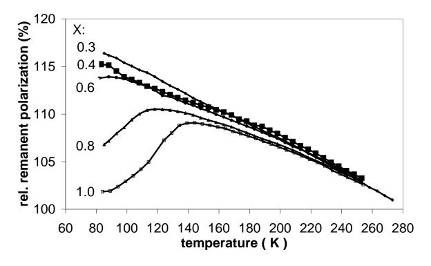
Open circuit remanent polarization of  $(Nd_xPr_{1-x})_2Fe_{14}B$  relative to the remanent polarization at 283 K, as a function of temperature, measured parallel to the alignment direction on samples of  $B/\mu_0H = -1.78(+/-0.04)$  for various x values. [2]
