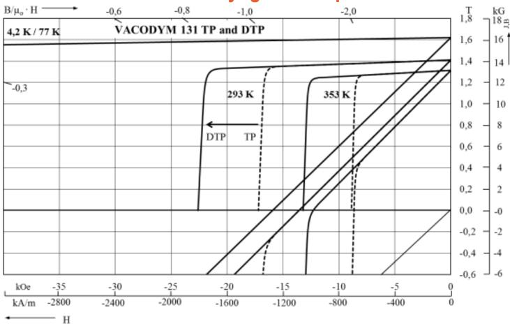
Demagnetization curves of VACODYM® 131 TP and DTP at cryogenic temperatures, room temperature and elevated temperature
